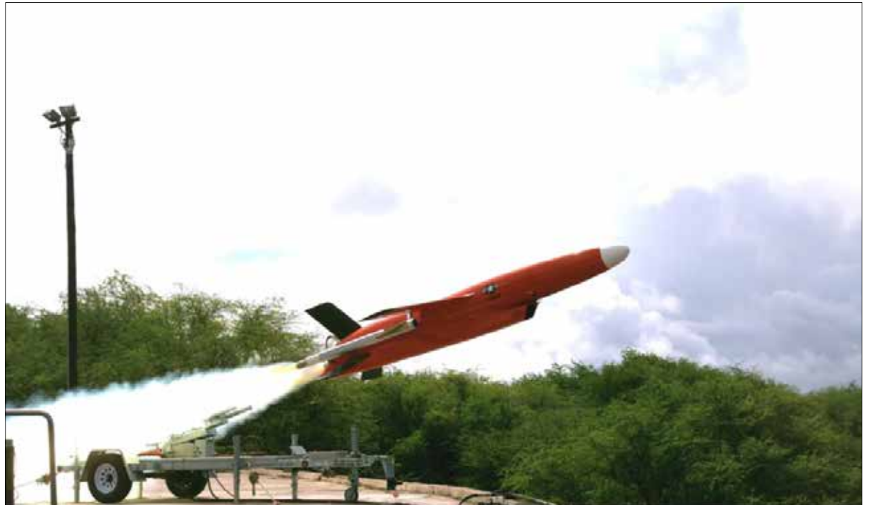
A BQM-177A Surface Launched Aerial Target takes to the air with the help of a Rocket-Assisted Takeoff attachment kit. Photo courtesy Kratos Defense
